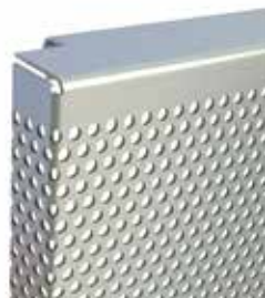
RV 3-5 Perforation percentage: min. 29 %, max. 31 % depending on panel width Perforation diameter: 3 mm
